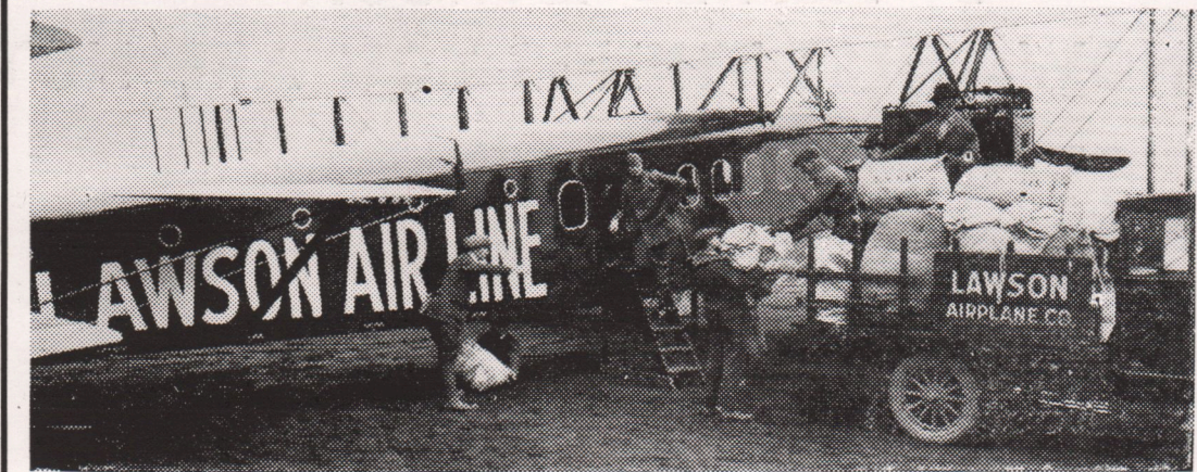
This is a photograph of Lawson's great AIRLINER built in the year of 1920 to carry 6,000 pounds of mail at a time. It was constructed so that mail could be routed within the cabin and transferred through a chute to a small Airplane from an aperture in the bottom of the cabin while in flight. Passengers could also be transferred in mid-air by the same method.
